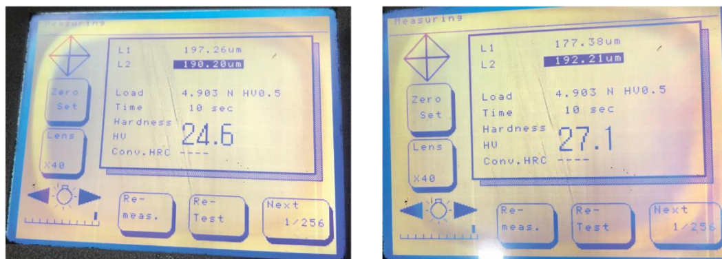
Figure 11: Vicker hardness Testing of Composite Material
