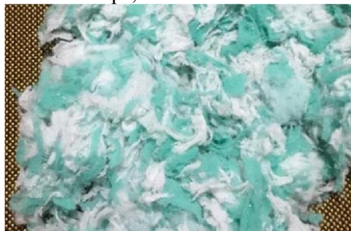
Figure 6: Shredded Polypropylene Fibers from Collected Face Masks
